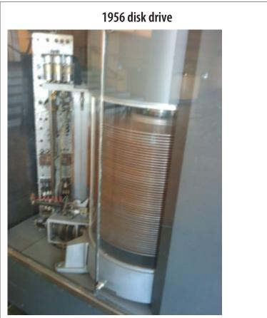
One of the first commercial disk drives from IBM. It has a 5 MB capacity and it's stored in a cabinet roughly the size of a luxury refrigerator. In contrast, a 32 GB microSD card measures around  $5/8 \times 3/8$  inch and weighs about 0.5 gram.
